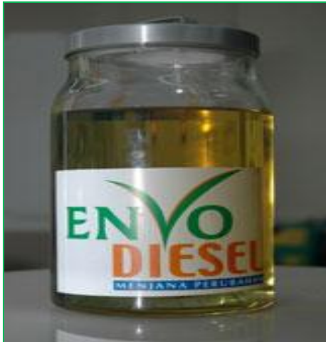
Palm Methyl Ester 100% concentration before it is blended with diesel and sold at petrol stations in Malaysia.
