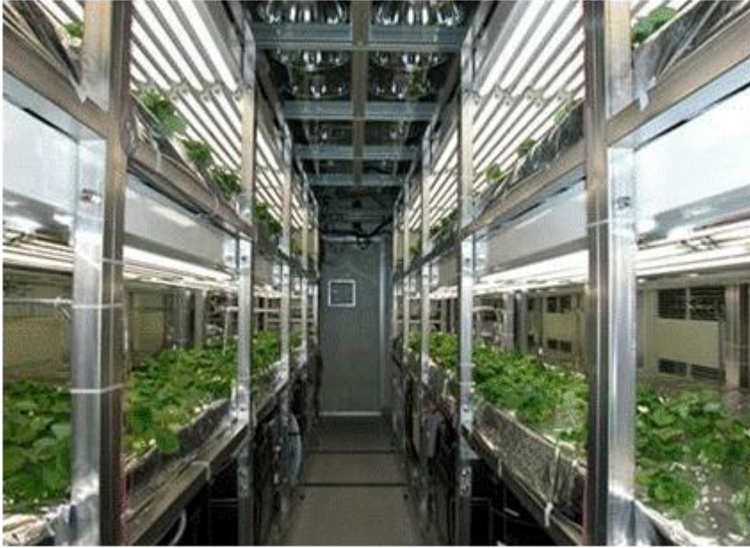
Figure; Closed-type transgenic plant production system for production of plant-made pharmaceuticals (National Institute of Advanced Industrial Science and Technology, http://www.aist.go.jp/aist_e/aist_laboratories/lifescience/index.html ).
