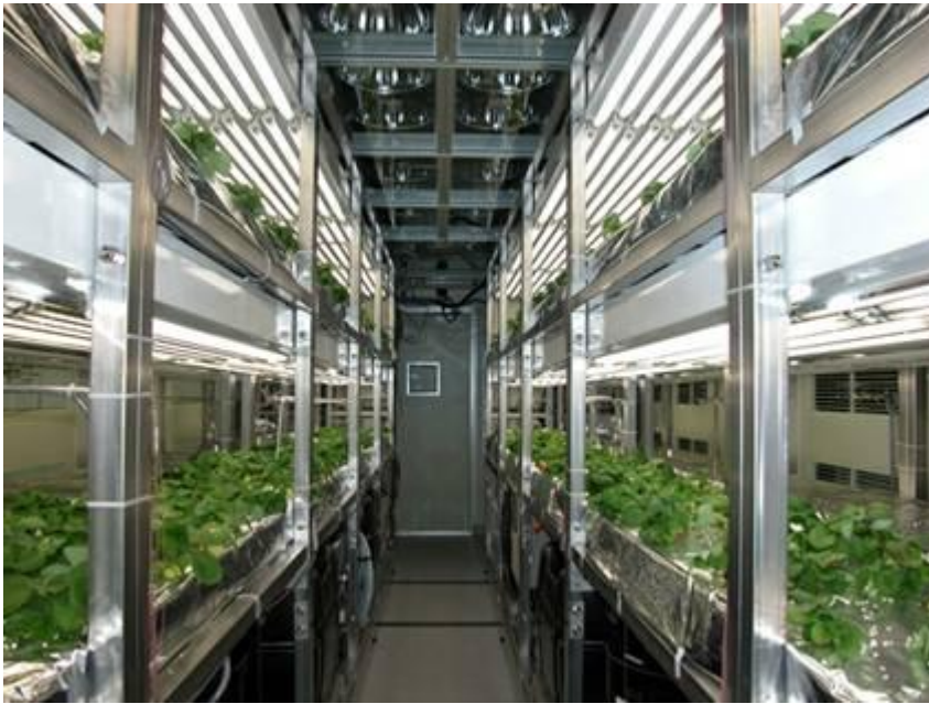
Figure; Closed-type transgenic plant production system for production of plant-made pharmaceuticals (National Institute of Advanced Industrial Science and Technology,
