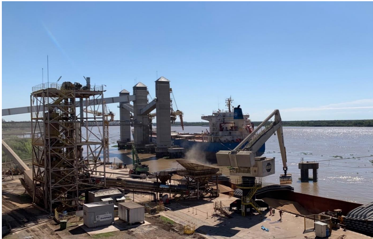
In foreground unloading barges of soybeans from Paraguay, in background loading soybean meal for export in ocean going vessel. Timbues, Santa Fe, April 2022 – Source: FAS Buenos Aires
