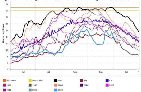
Figure 2: Mekong River Water Level Monitoring at Kratie Station
