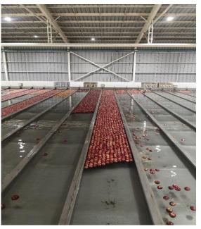
Apples are categorized automatically by size and color, before moving forward to the packing process.
